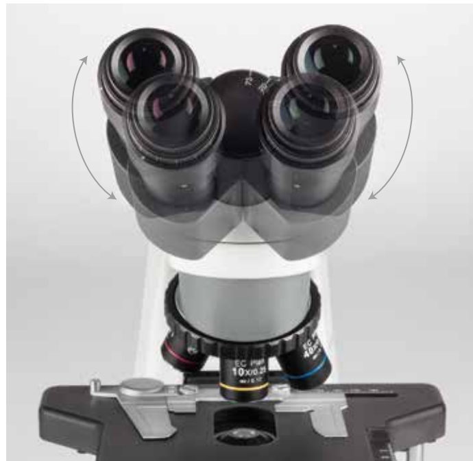
EYEPIECE TUBES | Interpupillary distance adjustment
